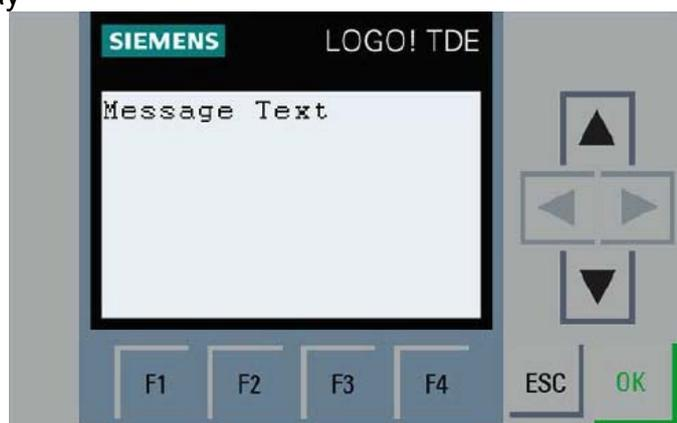
The TD is located on the door of the switchboard. It displays alarms and pressure, temperature and operating values. It has four cursor buttons ▲, ▼, ►, ◀ and the ESC and OK buttons. It also has four functional buttons, F1-F4, to control specific functions:
